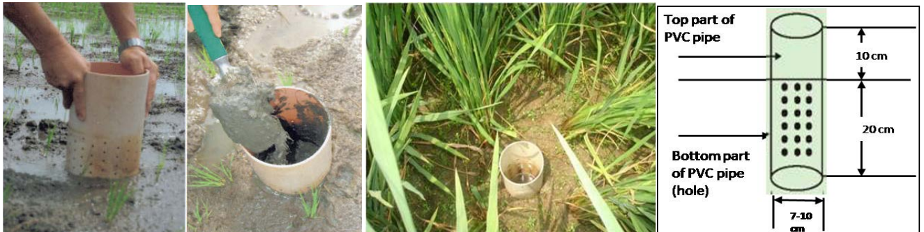
Fig. 2. AWD device installed in the soil
